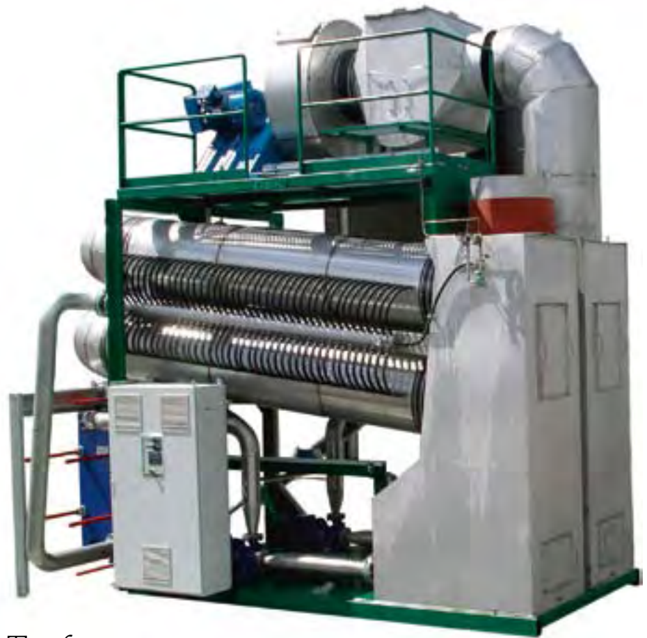
The condenser in SRE Renergi
